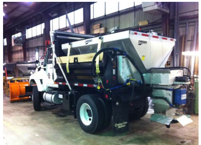
Dump Truck with Plow and Spreader
